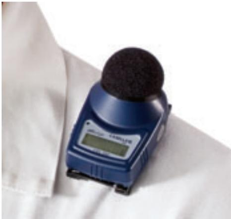
CEL-350 mounted on a shoulder using CEL-6351
