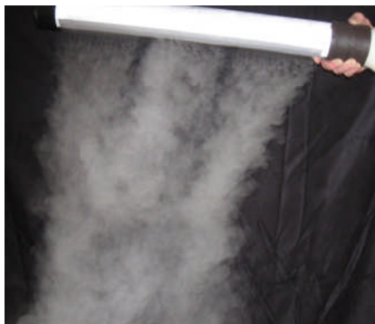
Optional Fog Curtain Wand to create a Wall of Fog to Visualize Airflow / Turbulence
